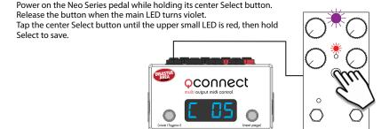
Power the Neo Series pedal off and back on, again holding the center Select button until the upper LED turns violet.
