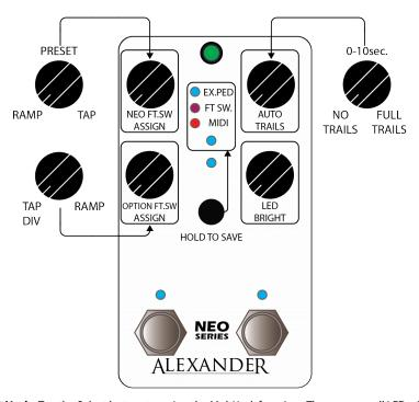
**MultiJack:** Tap the Select button to assign the MultiJack function. The upper small LED will light to indicate the function.
