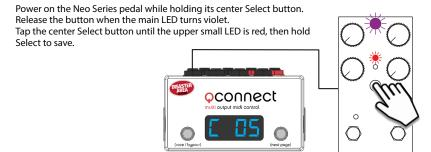
Power the Neo Series pedal off and back on, again holding the center Select button until the upper LED turns violet.
