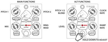
**DYNA** (upper violet) Dynamically controlled pitch shifter. VOICE sets the "quiet" interval and TWO sets the "loud" interval. Adjust MOD to control the sensitivity of the envelope detector. ALT sets the shift behavior to either glide between pitches or smoothly fade.
