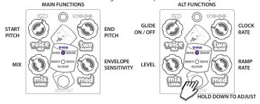
**CLOUD** (lower violet) Twin pitch shifters with an adjustable cascading delay / reverb effect. Increase the MOD knob for more clouds, lower the CLOCK knob for longer delays.
