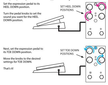
Just like with the WARP footswitch, all of the knobs on the pedal can be controlled with the expression pedal except RAMP RATE, PITCH LOCK, and the mode selection.
