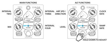
**RAND** (upper red) Twin pitch shifters with random modulation. VOICE and ALT set the "home" pitches of each shifter and MOD sets how far they're allowed to move.
