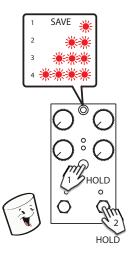
To save the current preset, press and hold the center Select button, then hold the BYPASS footswitch down.
