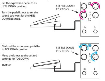
All of the knobs on the pedal can be controlled with the expression pedal except the mode selection.
