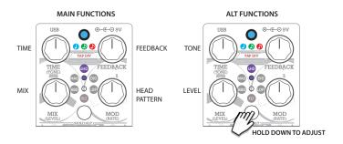
**FLT** (lower violet) 12-bit rack-style digital delay. TONE controls a resonant filter, and MOD adds a pitch detune for thickening or wild modulation effects.
