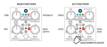
**4HD** (upper violet) Four-head multi-tap delay. TONE controls the brightness of the echo signal, and MOD selects one of eight head patterns.
