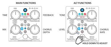
**DIG** (upper red) Bright and clean 24-bit digital delay. MOD and RATE control a digital pitch modulator, and TONE pans between bright and dark voicings.
